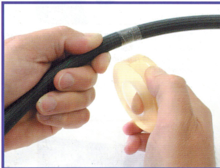
1. Measure desired hose length and wrap tightly with AeroFlow's non-stick cutting film, (part # AF98-2049), allowing at least 3 full rotations of the non-stick film.
