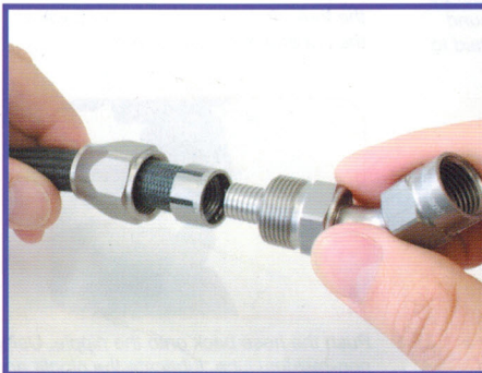
5. Carefully slide olive past non-stick film then remove the non-stick film and slide olive back up to end of hose. Apply a small amount of Aero-Seal (part # AF98-2023), onto the male thread of the Kryptalon® hose end and screw the socket nut onto the Kryptalon® hose end.
